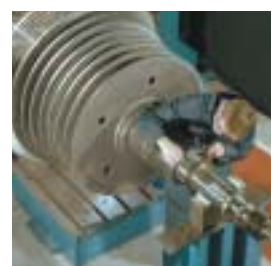
2 LP stages of a 6MW Daniel Adamson turbine being manufactured for a UK fertiliser plant.
