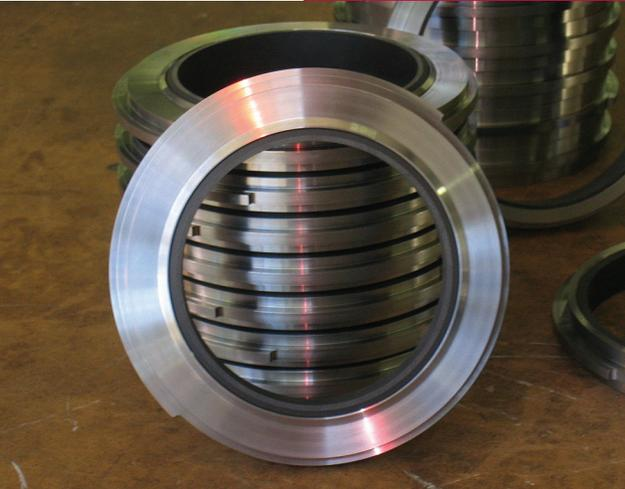
Fluid processing industries have embraced the use of composite materials in pumps to reduce vibration, increase mechanical seal life and MTBR (mean time between repair), reduce the risk of seizure, increase efficiency, and reduce repair costs. API 610, 10<sup>th</sup> Edition (ISO standard 13709), the latest centrifugal pump standard from the American Petroleum Institute (API), recognizes the use of composites to achieve these benefits.
